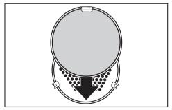
The roasting filter must be fitted in front of the fan when cooking anything fatty or where food is likely to splatter, e.g. when open roasting or grilling meat. The droplets of fat caught up in the circulating air are deposited on the roasting filter. This helps to keep the oven and the area behind the interior back panel cleaner.
